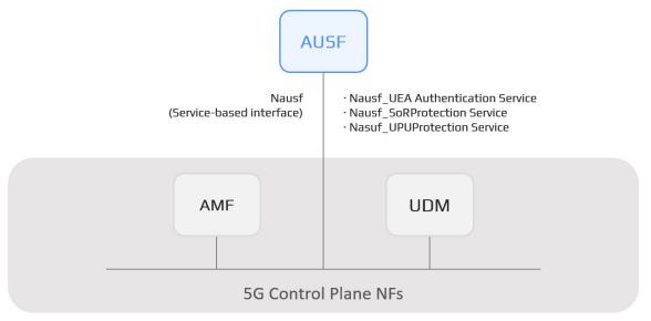
[Fig. 1] AUSF Non-Roaming Architecture
