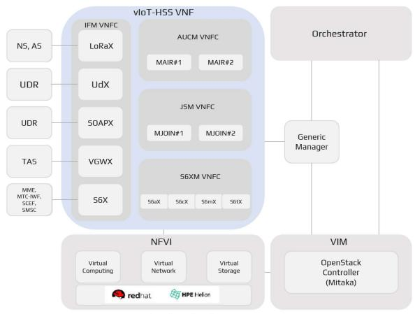
[Fig. 2] NFV-based IoT-HSS FE structure
