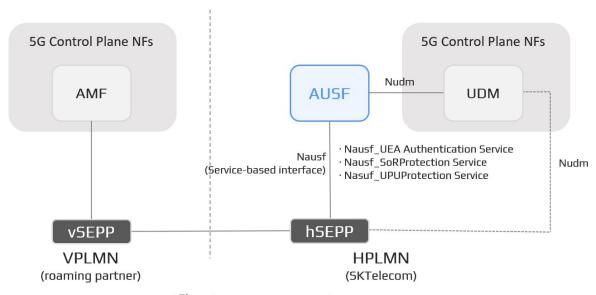
[Fig. 2] AUSF Roaming Architecture
