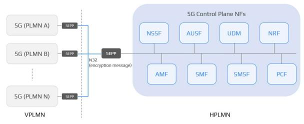
[Fig. 1] SEPP Network Architecture
