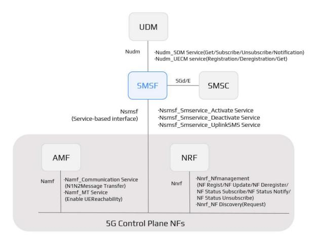
[Fig. 1] SMSF Network Architecture
