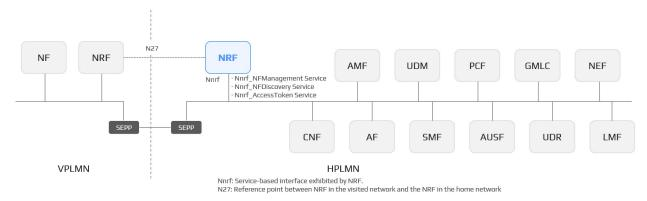
[Fig. 1] 3GPP 5G System Architecture-based NRF Interconnection Interface
