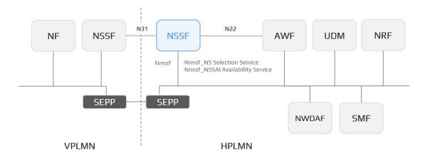
Nnssf: Service-based interface exhibited by NSSF N22: Reference point between AMF and NSSF
