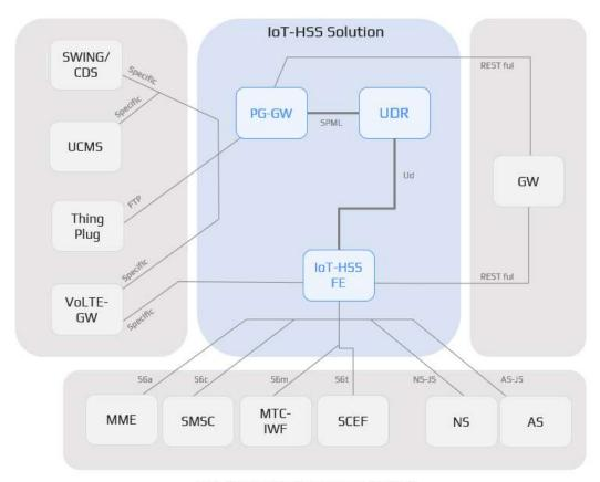
[Fig. 1] IoT-HSS solution components
